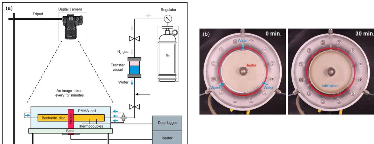
**Fig. 1** (a) Experimental setup and (b) photographs taken at 0 and 30 minutes after the start of water infiltration showing the bentonite turning dark with saturation
